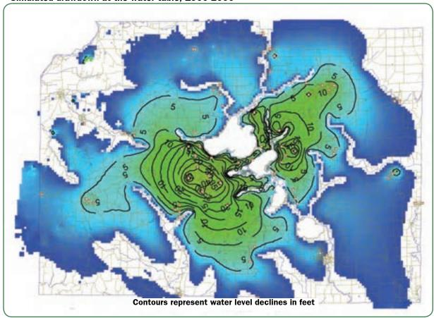
Figure 18 Simulated drawdown at the water table, 2000-2030
