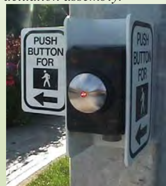
Above: Solar LED flashing beacon. Below: User actuation assembly.
